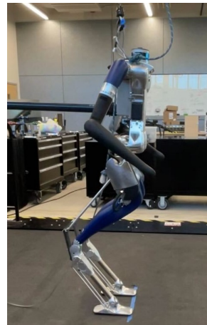
Fig. 1: The experimental setup that was used to collect hardware data with the Digit robot [1].
